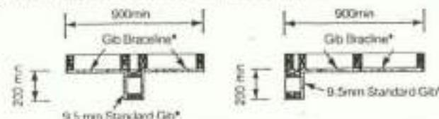
Where Wall Bracing Elements are interrupted by T or L junctions (as illustrated in the 900mm example above) they should be considered as follows: The Gb Braceline\* has been cut to accommodate the junction. Nevertheless, in respect of calculating Bracing Units, the Bracing Element is deemed to be continuous for the whole length (900mm in this particular case).
